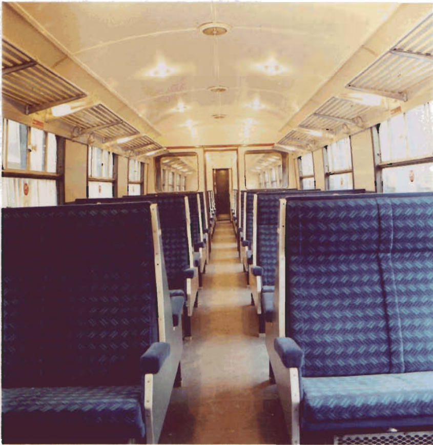
Fig 8. An interior view of Mark 1 rolling stock similar to some carriages of the Poole train, showing lateral luggage racks.
